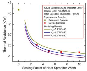
Figure 4, Experimental data of the thermal resistances of GaAs samples with different heat spreader widths. Reference sample is included for comparison. Three curves from analytic modeling are also plotted. Different thermal conductivity values of  $Si_3N_4$  are used to fit the experimental data.
