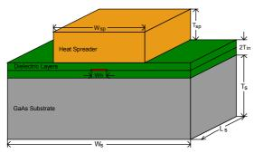
**Figure 1**, Schematic illustration of the test structure used for evaluating the effectiveness of the integrated heat spreaders for high power semiconductor lasers. The meander-shaped microheater stripe is embedded between two dielectric layers. High thermal conductivity copper is deposited on top of the structure to serve as heat spreader.
