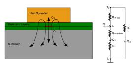
**Figure 6**, Two-dimensional analytical model for the test heat spreader structure. Left: two-dimensional structure picture of the test sample; right: thermal circuit for the calculation of the thermal resistance of the test sample.
