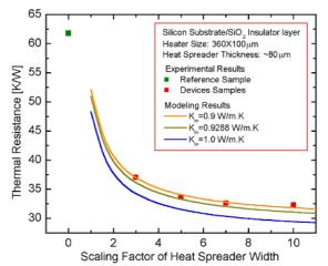
**Figure 5**, Experimental data of the thermal resistances of Si samples with different heat spreader widths. Reference sample is included for comparison. Three curves from analytic modeling are also plotted. Different thermal conductivity values of SiO<sub>2</sub> are used to fit the experimental data.  $K_{in} = 0.9288W/m \cdot K$  is determined by fitting the thermal resistance of the reference sample with the analytical model result.
