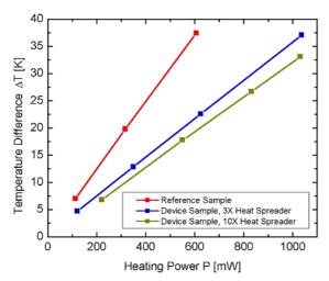
**Figure 3**, Temperature difference  $\Delta T$  between heaters and sample bottom surfaces as a function of heating power P. Experimental data are from Si samples with SiO<sub>2</sub> as dielectric layers (heater:  $360\mu m \times 100\mu m$ ; copper heat spreaders thickness:  $80\mu m$ ).
