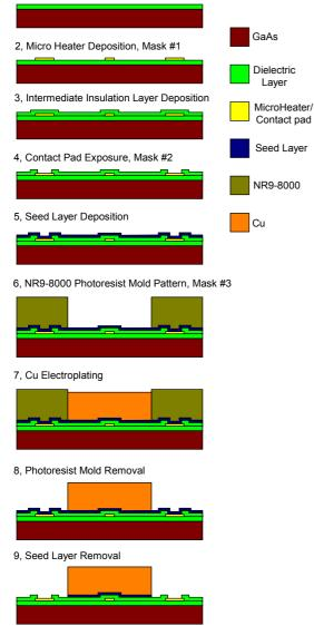
Figure 2, Fabrication process flow of the integrated copper heat spreader structure.
