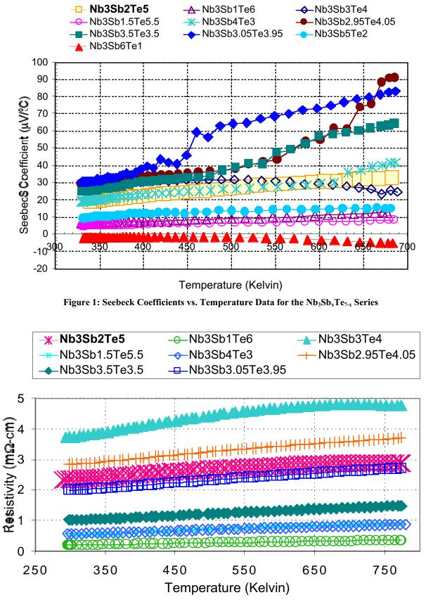
Figure 2: Resistivity vs. Temperature Data for the Nb<sub>3</sub>Sb<sub>x</sub>Te<sub>7-x</sub> Series
