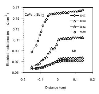
Figure 4. Electrical contact resistance as a function of distance for a p-CeFe $_4$ Sb $_{12}$ /Nb junction using a Cu $_2$ Ag $_{72}$  alloy interface. The origin corresponds to the interface position.
