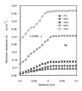
Figure 3. Electrical contact resistance as a function of distance for a n-CoSb $_3$ /Nb junction using a Cu $_{28}$ Ag $_{72}$  alloy interface. The origin corresponds to the interface position.
