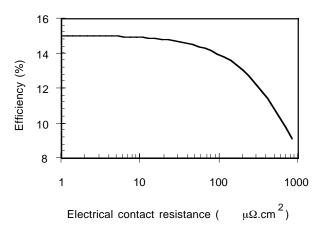
Figure 2. Thermoelectric efficiency as a function of electrical contact resistance (the same contact resistance was taken for each of the junctions in the calculations).
