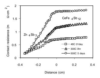
Figure 7. Electrical contact resistance as a function of distance for a p-CeFe $_4$ Sb $_{12}$ /p-Zn $_4$ Sb $_3$  junction using a Pd $_{70}$ Ag $_{30}$  alloy interface. The origin corresponds to the interface position.
