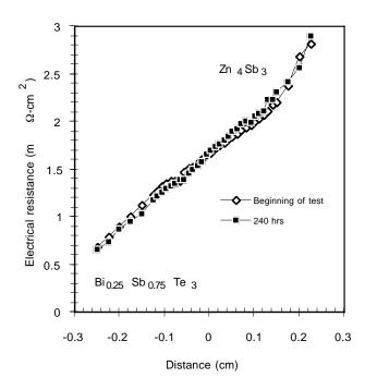
Figure 5. Electrical contact resistance as a function of distance for a p- $Zn_4Sb_3/p$ - $Bi_{0.25}Sb_{0.75}Te_3$  junction using a Pd interface. The origin corresponds to the interface position. The test was conducted at 150°C.
