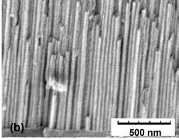
**Figure 1**. Template made by anodizing a 10  $\mu$ m thick layer of aluminum on silicon, with pore diameter 12 nm. (a) top view; (b) cross section.
