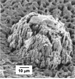
**Figure 2.** Bi<sub>2</sub>Te<sub>3</sub> nanowires, 200 nm diameter, grown in a 50 μm bundle. The alumina template has been etched away.
